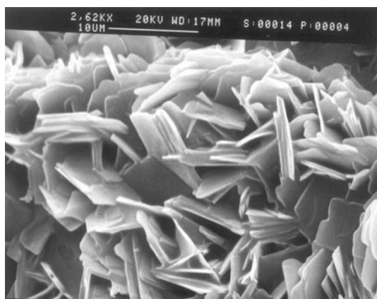
Fig. 13 SEM photograph of GW468816E melted and then heated up to 152 °C in the DSC cell
